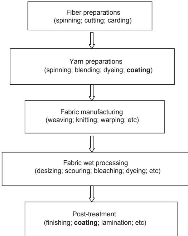
**Figure 1.1** Coating positions in textile processing.
